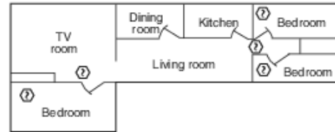
FIGURE A.29.5.1(c) In Dwelling Units with More Than One Sleeping Area, Smoke Alarm Should Be Provided to Protect Each Sleeping Area in Addition to Smoke Alarms Required in Bedrooms.
