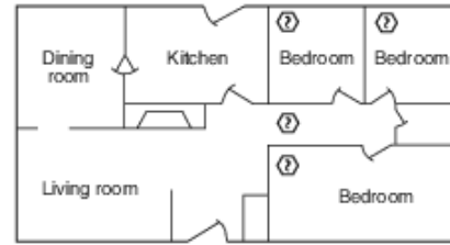
FIGURE A.29.5.1(b) Smoke Alarm Should Be Located Between Sleeping Area and Rest of Dwelling Unit, as Well as in Each Bedroom.
